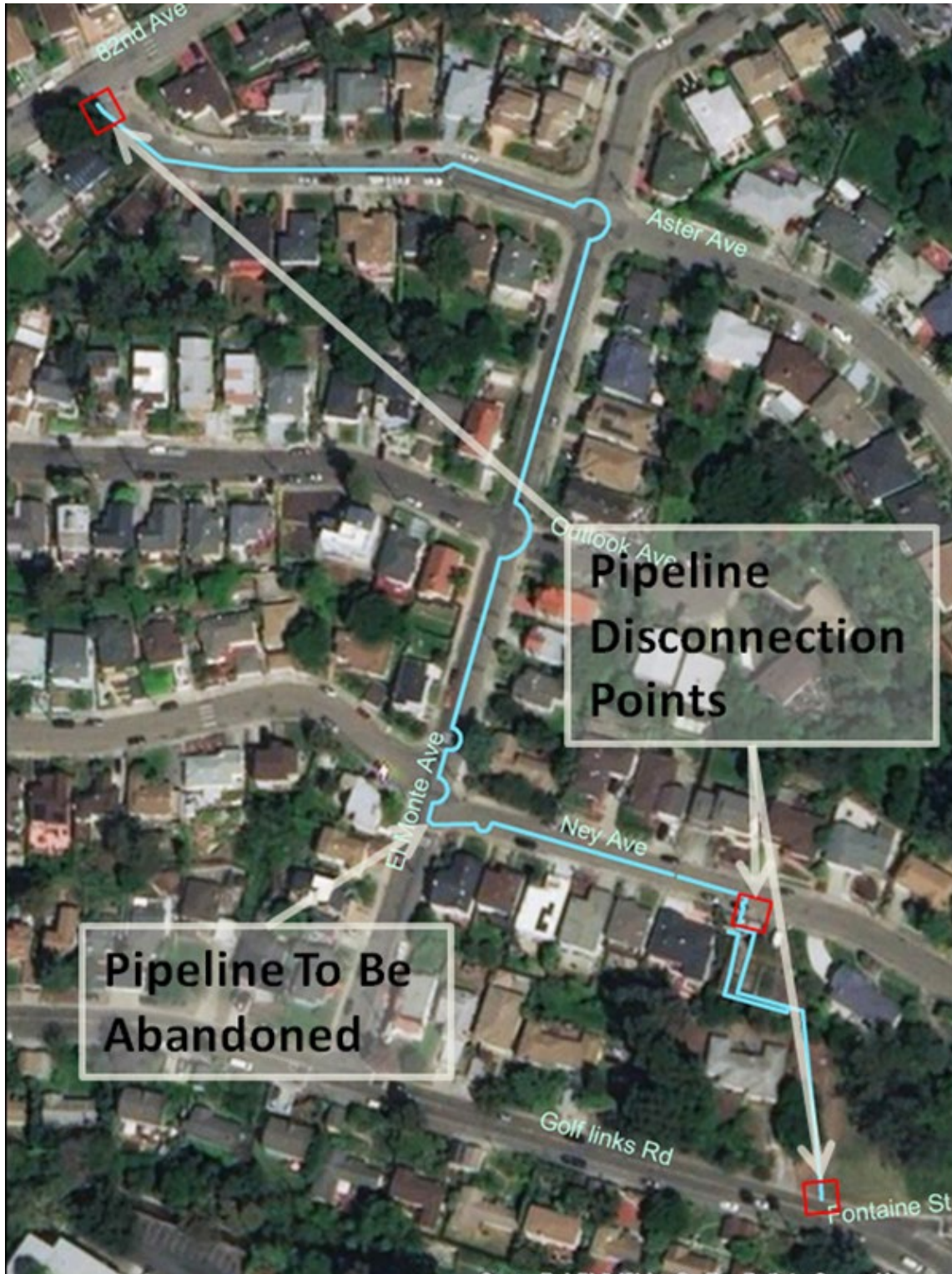
Figure 2 Existing Pipeline Abandonment Disconnection Sites
