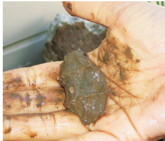
Soil forms a “cast,” an impression of your fingers. Photo: Josh Lowe.
