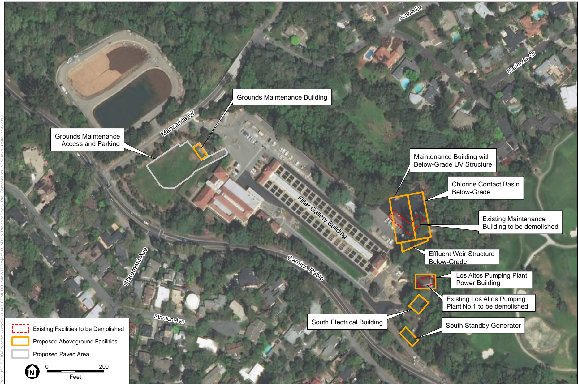
Figure ES-2 Proposed Project Components on Existing Orinda Water Treatment Plant Site
