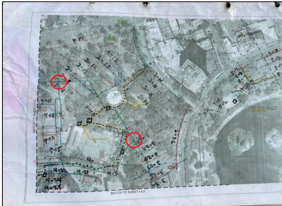
Customer provided “As-Builts” with closed isolation valves
