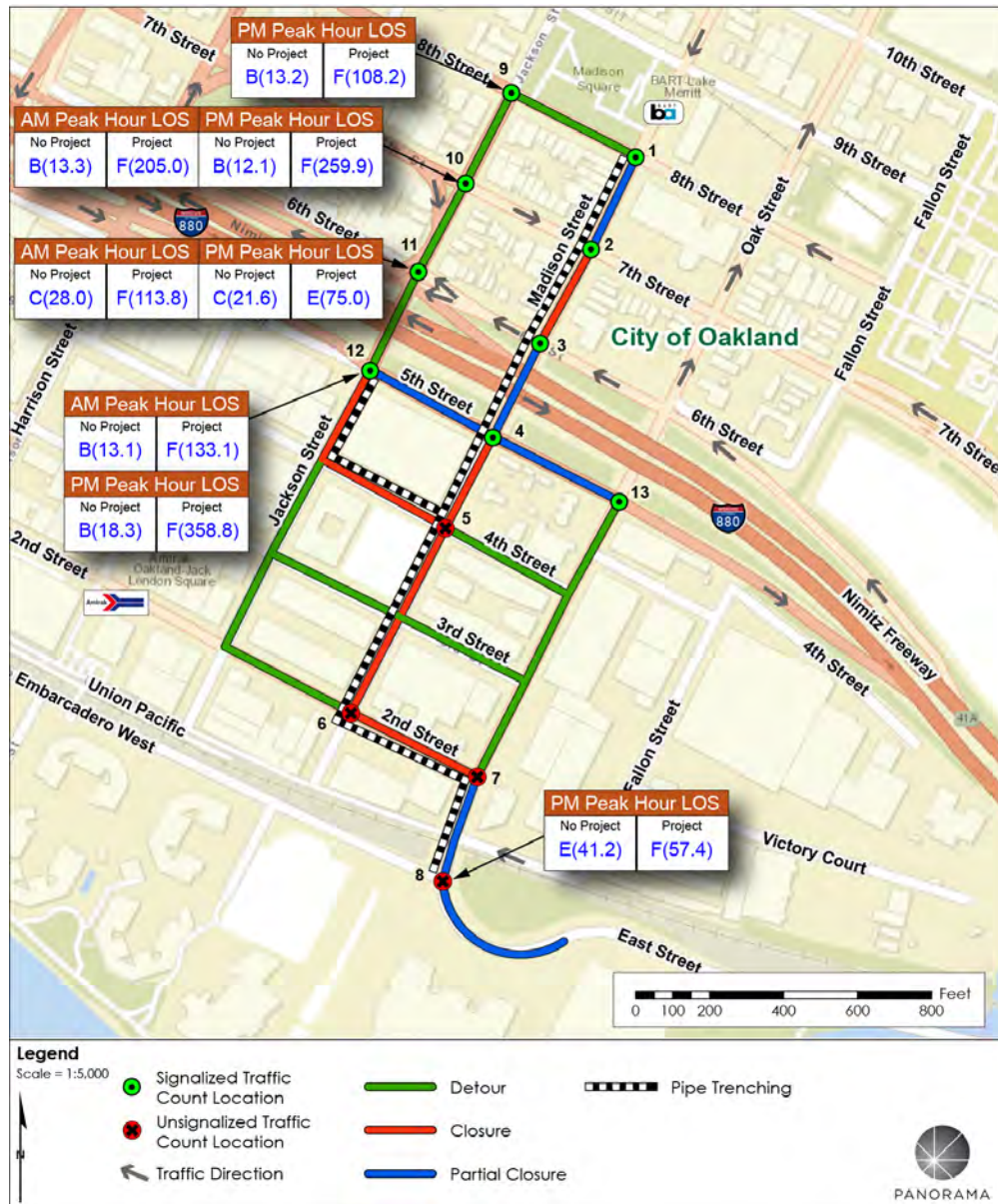
Figure 15 Full & Partial Closure & Detour Routes (Oakland Crossing #1)
