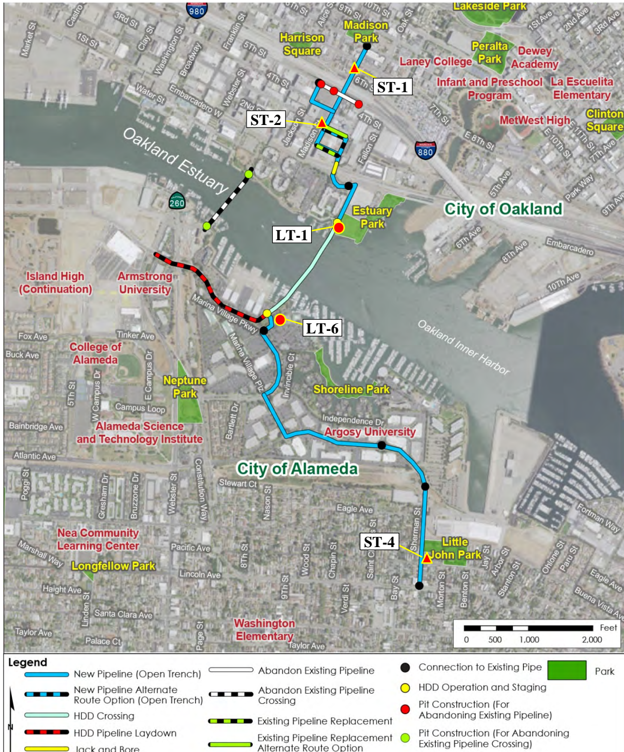
Figure 5 Crossing #1 Alignments and Measurement Locations
