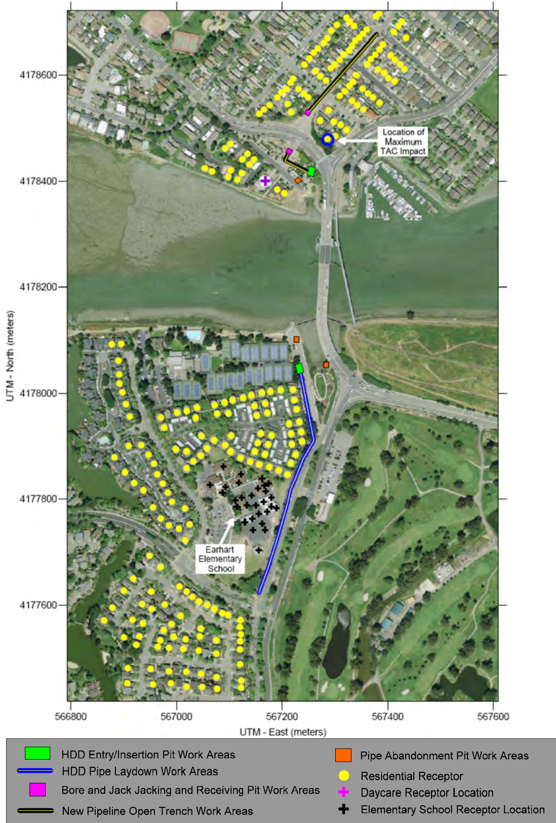
Figure 8: Crossing #2 - Project Areas, Sensitive Receptor Locations, and Location of Maximally Exposed Individual
