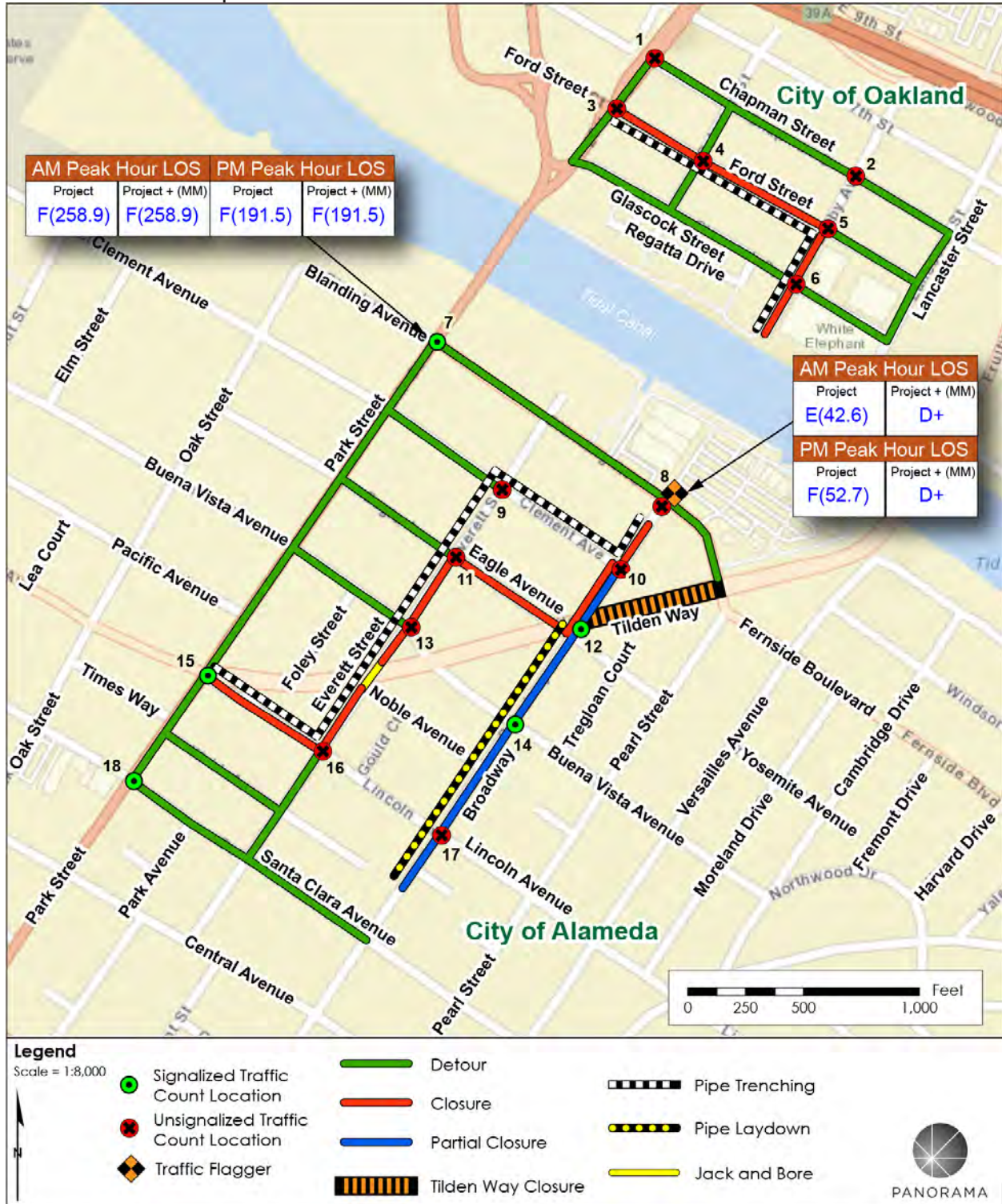
Figure 23 Full & Partial Closure & Detour Routes (Oakland & Alameda Crossing #3) For Alternate Trench Option
