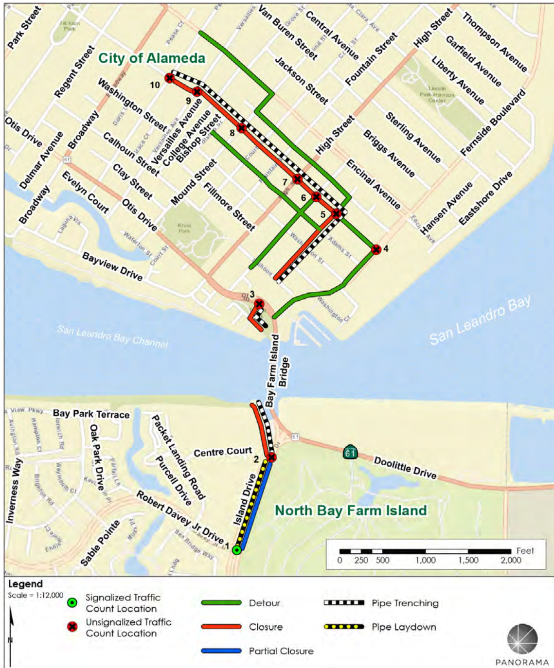
Figure 18 Full & Partial Closure & Detour Routes (Alameda Crossing #2)
