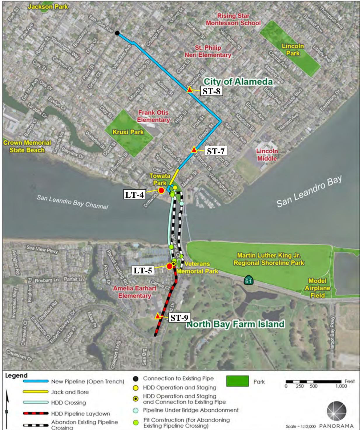
Figure 6 Crossing #2 Alignments and Measurement Locations
