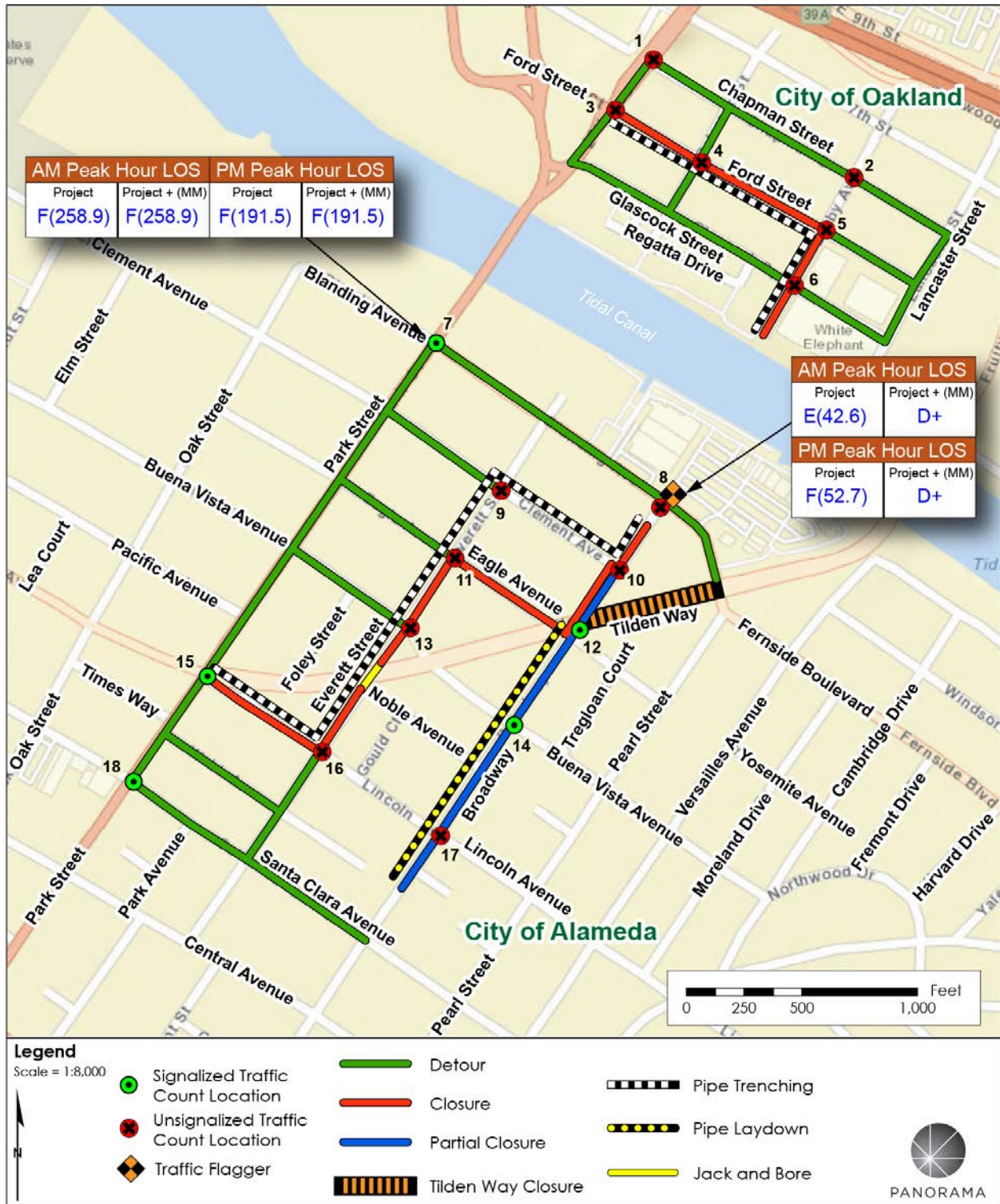
Figure 3.13-7 Road Closures and Detours for the Alternate Route Option for Crossing #3 after Mitigation
