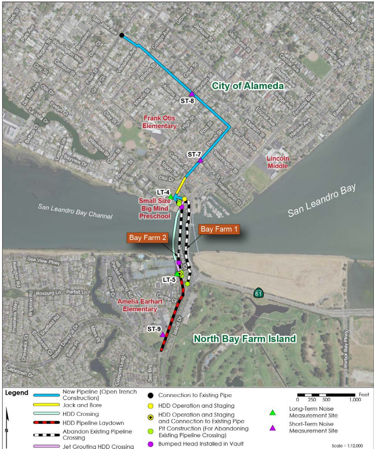
Figure 3.11-2 Noise Survey Locations and Sensitive Receptors (Crossing #2)
