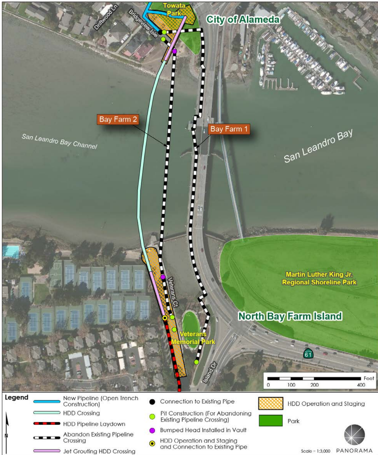
Figure 2.1-4 Detail of Crossing #2 Alignment
