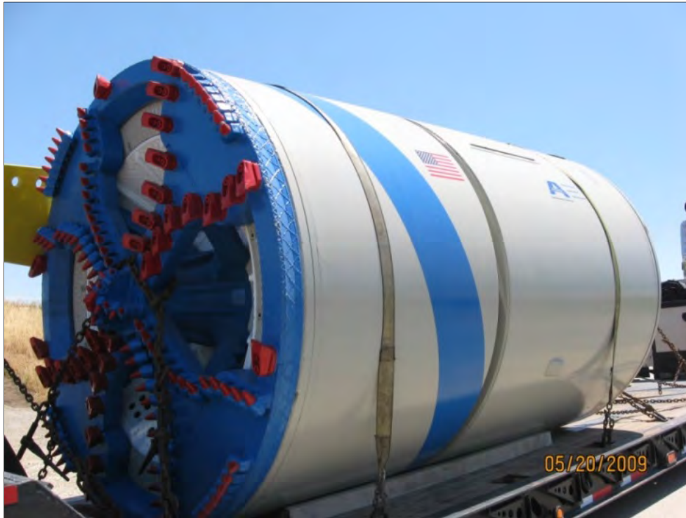
Figure 4-1. Typical Microtunnel Boring Machine (MTBM)
