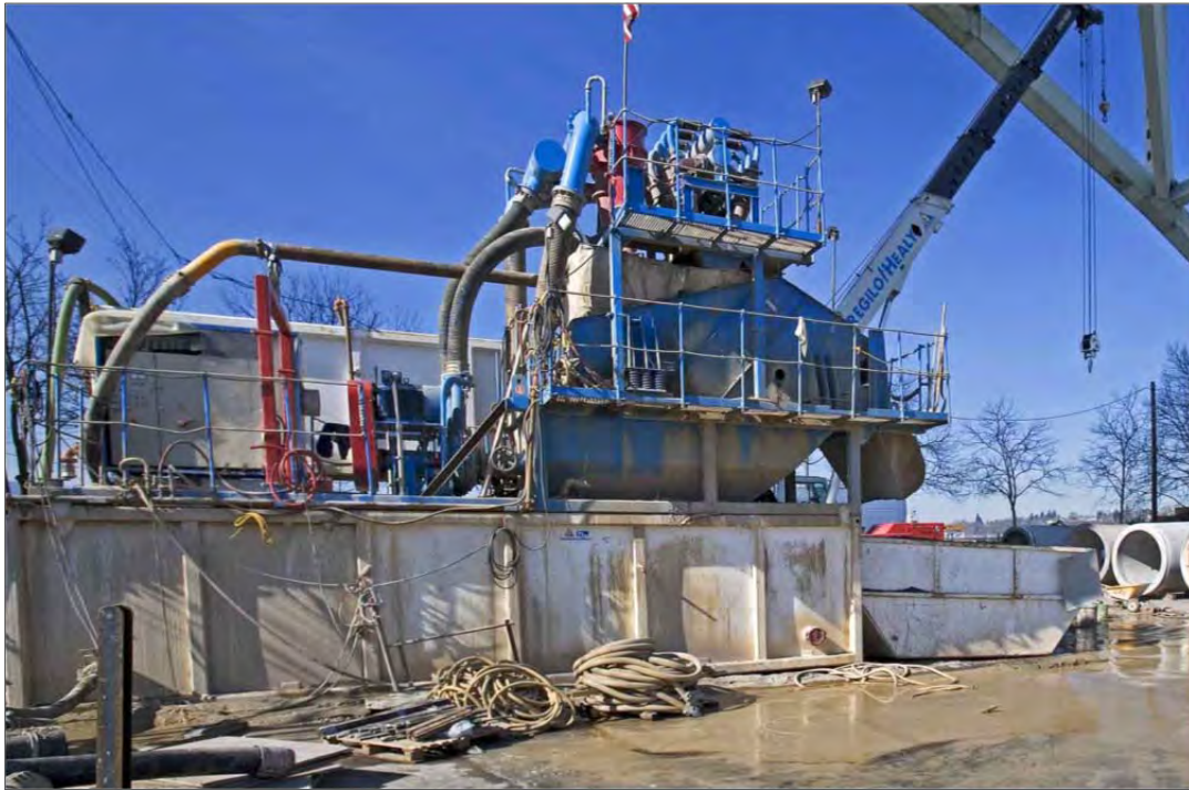
Figure 4-3. Typical Slurry Separation Plant
