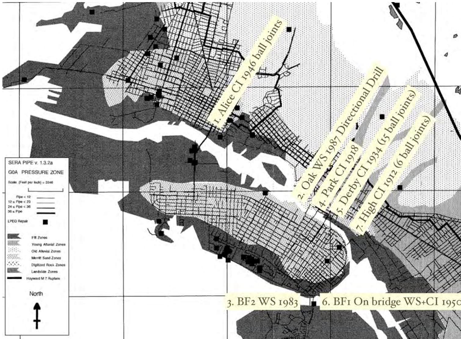
Figure 1-3. Existing Pipeline Crossings: Type of Construction and Age of Original Installation (grid lines are at 10,000-foot intervals)
