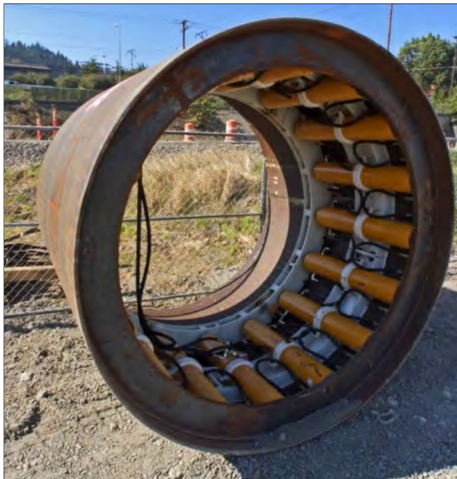
Figure 4-4. Intermediate Jacking Station (IJS)
