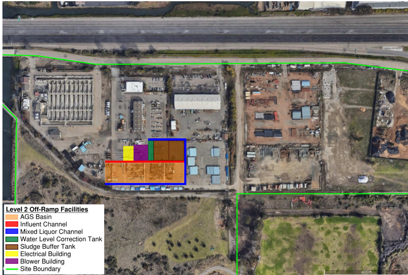
Figure 5-14. Alternative 6 Decentralized – Conceptual Site Layout for Oakport WWF
