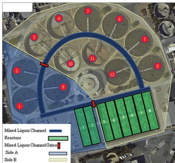
Figure A: East Bay Municipal Utility District Main Wastewater Treatment Plant layout and split-plant configuration. Side A and Side B operate at high and low mean cell residence times, respectively, during split-plant testing.
