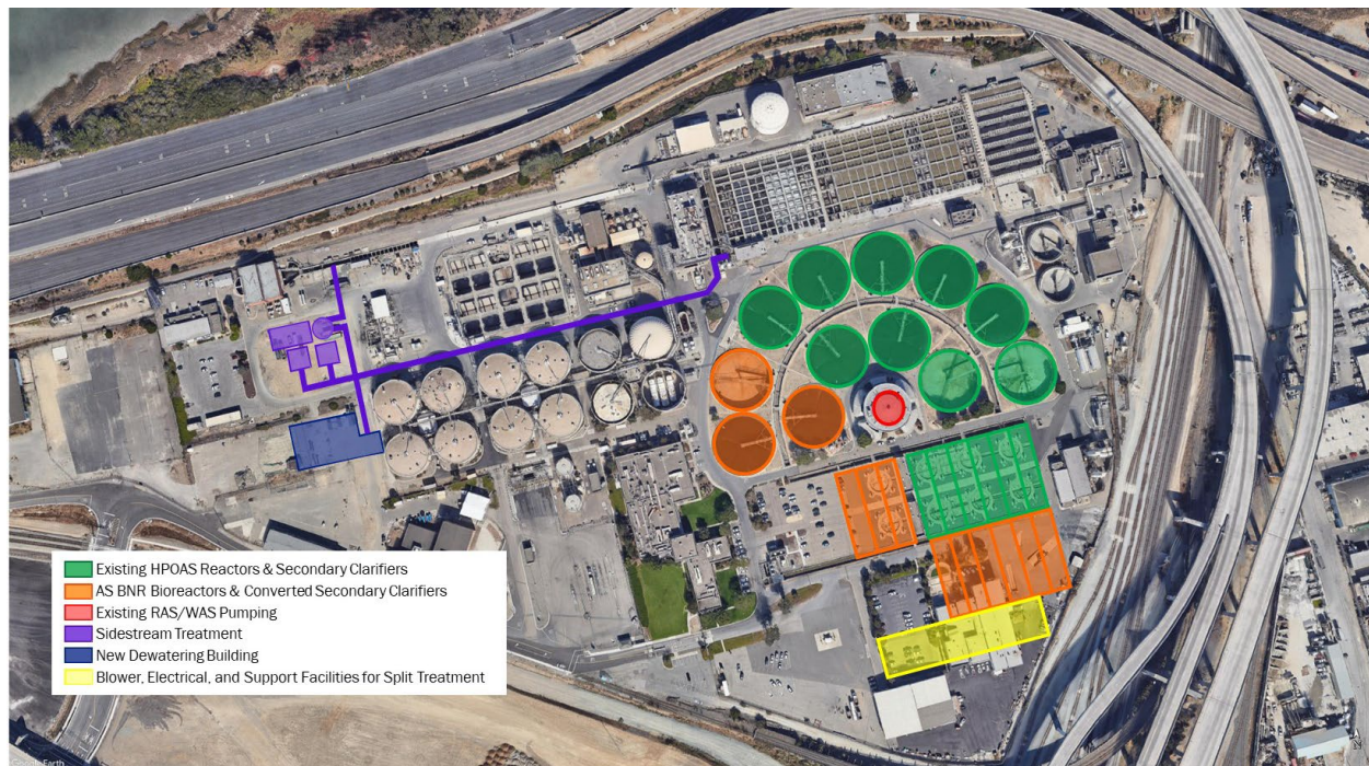
Figure 4-8. Site plan for SST and split treatment to meet the Master Plan Target beyond the planning horizon
