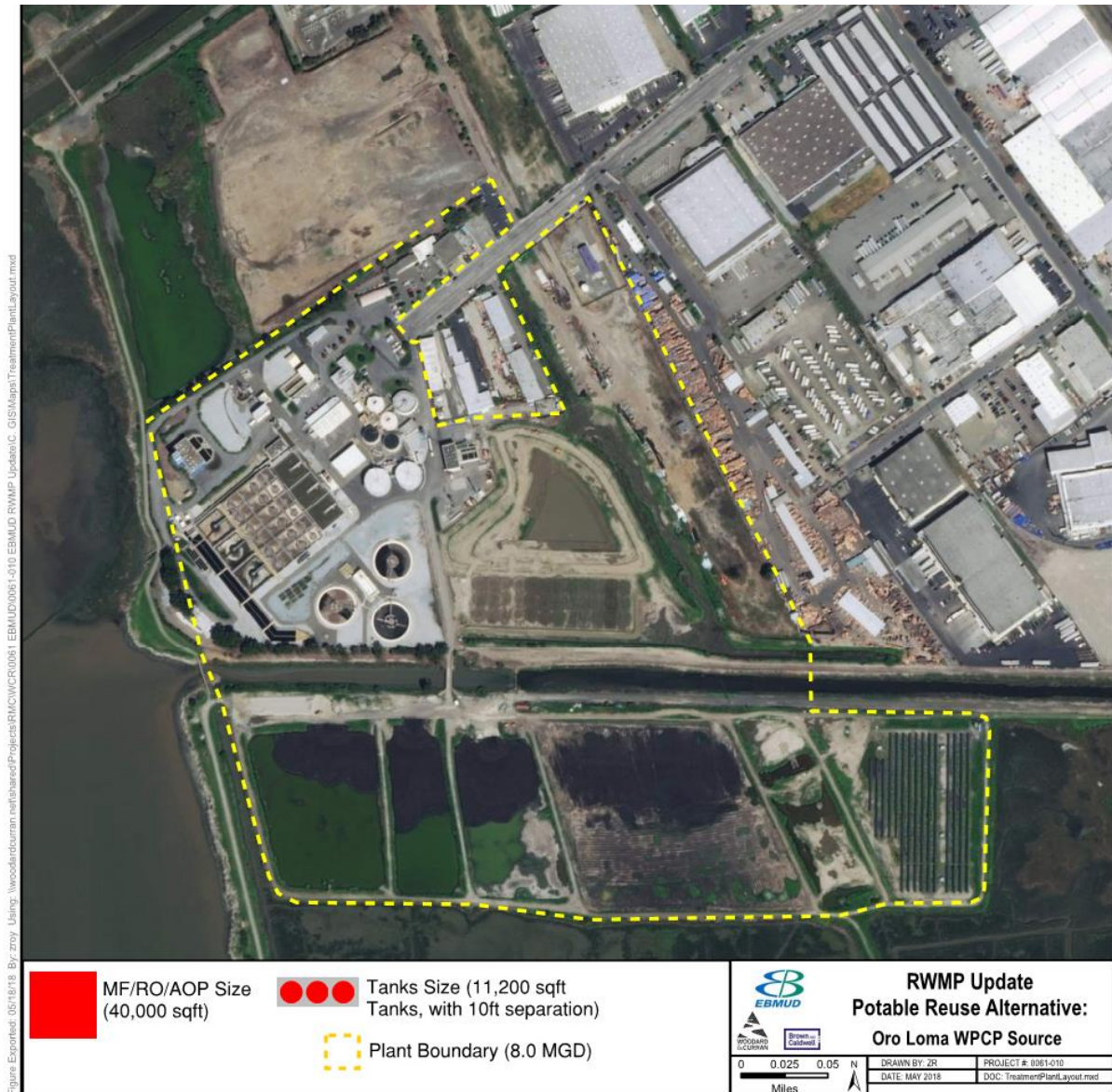
Figure 4-24: Advanced Treatment Footprint at Oro Loma WPCP
