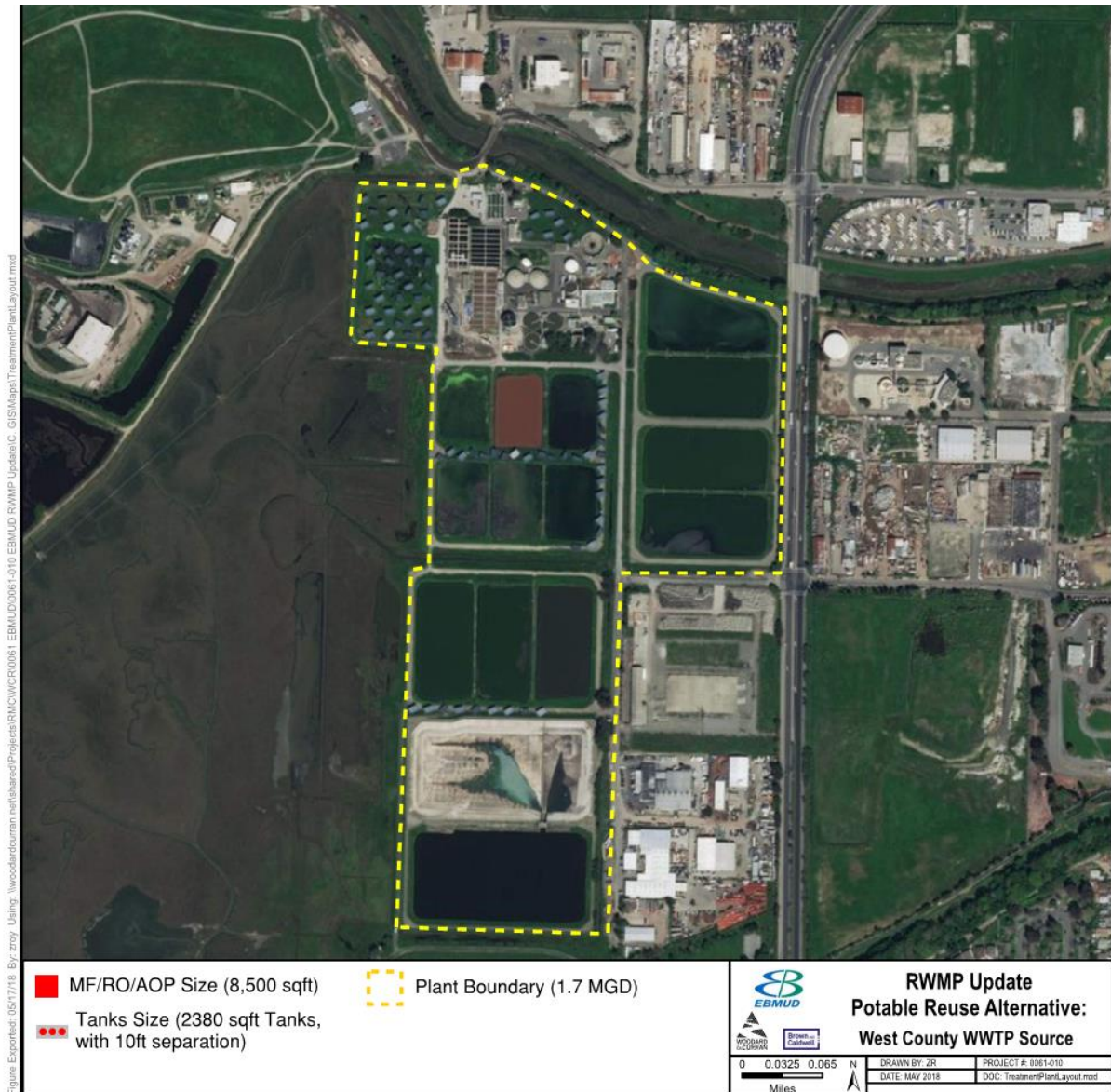
Figure 4-22: Advanced Treatment Footprint at West County WWTP
