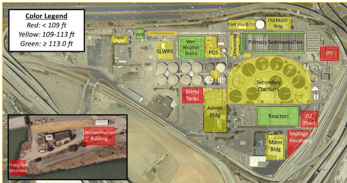
Figure 0-2. Elevation map of MWWTP structures
