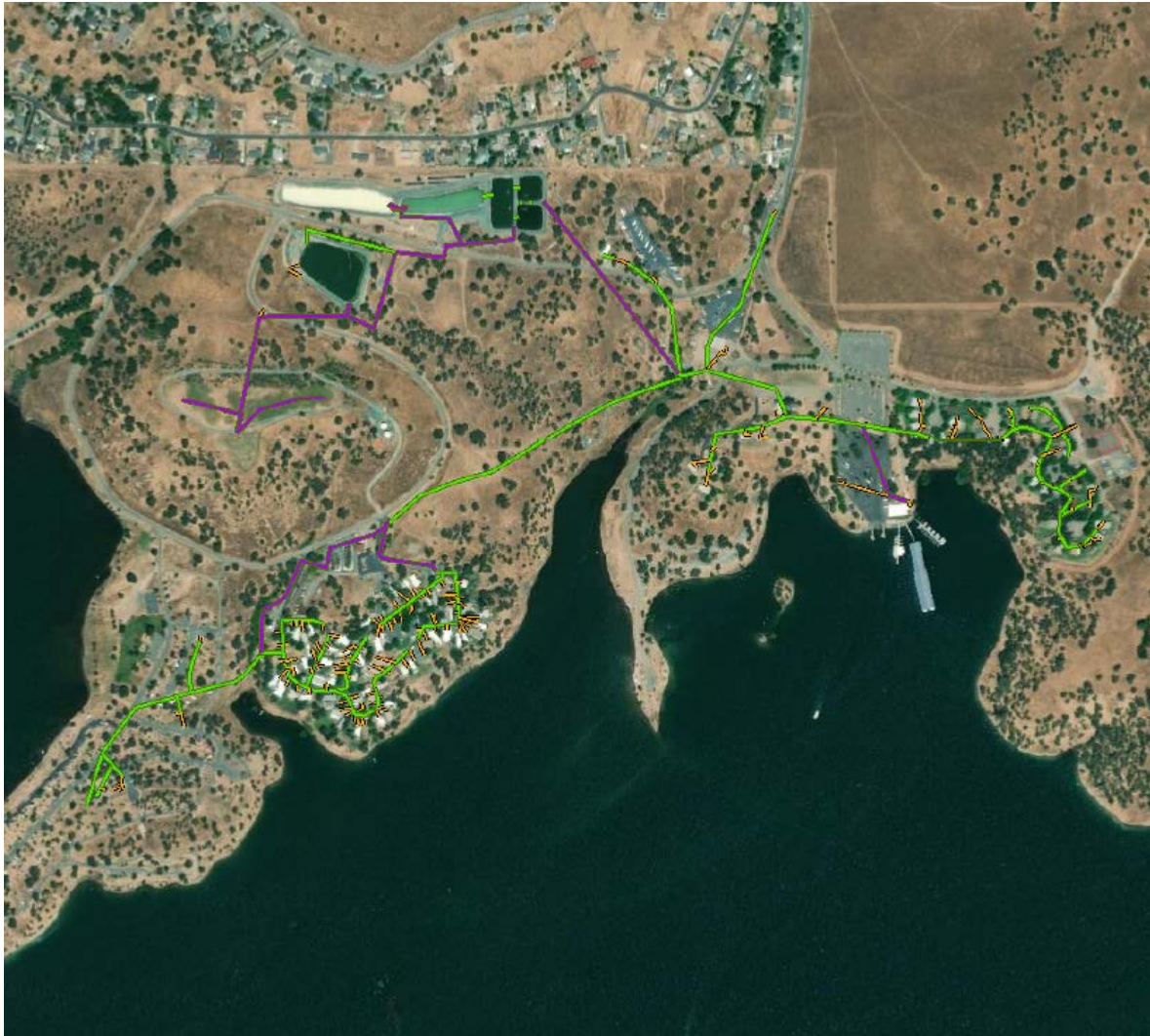
Figure 2 - CANS Wastewater System yellow lines = sewer laterals, green = sanitary sewer lines, and purple = force mains (including treated effluent discharge to spray-fields)
