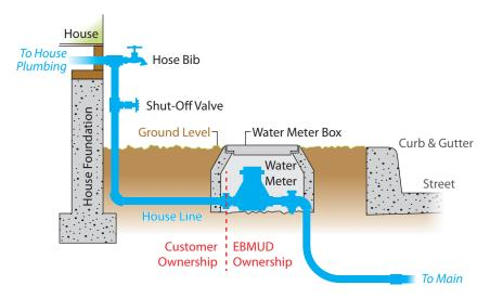
Your irrigation system might branch off before reaching your house line shut-off valve. If so, you may need to test both the irrigation pipes and the house line.
