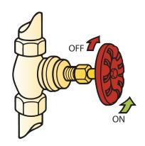
**Step 2** After you have turned off the house line shut-off valve, line up a toothpick or a pin with the hand of the meter or take a picture, as before. Wait 30 minutes, then look at the water meter dial.
