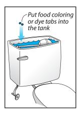
the toilet tank. A flapper test will tell you if the flapper valve is leaking. To complete a flapper test, you will need food coloring or dye tabs. Put enough food coloring in the toilet tank
