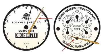
**Step 4** Wait for 30 minutes. Then, before turning on any faucets or hoses, check the dial of the meter to see if the hand has moved.
